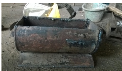
Gambar 4. Bak Galvanize (Crusible)
