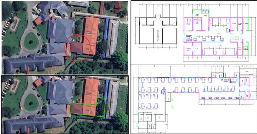
Figure 1. Building in red circle (top left image) is the existing Sri Pamela Hospital Hemodialysis Service Unit building. The L-shaped green line (bottom left image) is the planned expansion for the Hemodialysis Service Unit building. The top right image is the existing Hemodialysis Service Unit floor plan, while the one below it is the floor plan after the building expansion.
