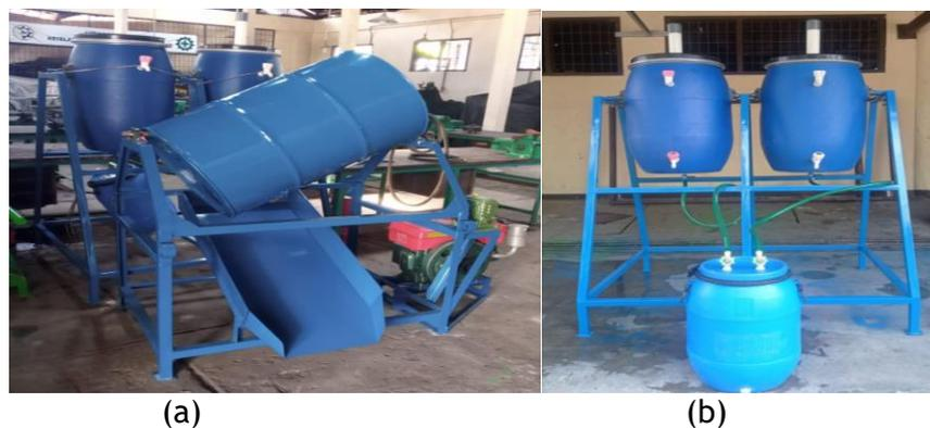
Gambar 2. (a) Rotary biocomposter, (b) Fermentor
