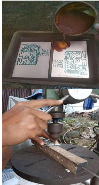
Gambar 2. Proses produksi PCB (printed circuit board) purwarupa SLIFA Connect
